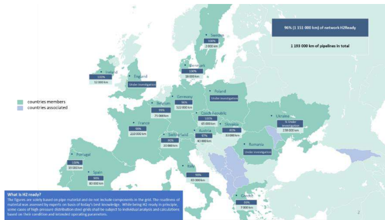
Figure 30: Readiness for pipeline's repurposing potential. Source: Ready4H2 146 .
