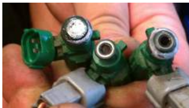
Corrosion in fuel injector caused by EBP
