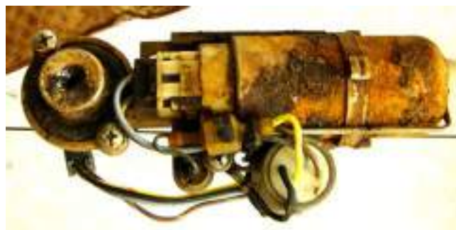
Corrosion in Fuel pump caused by EBP
