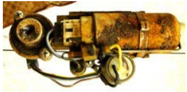
Corrosion in Fuel pump caused by EBP
