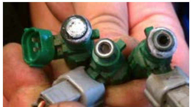
Corrosion in fuel injector caused by EBP
