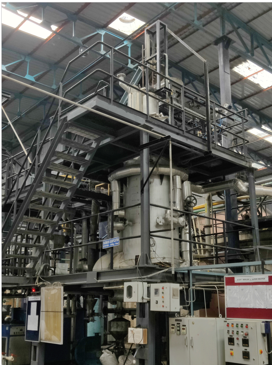
The oxy-steam gasification system at the Combustion, Gasification and Propulsion laboratory (CGPL), IISc
