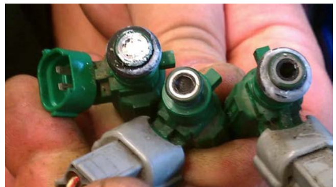
Corrosion in fuel injector caused by EBP
